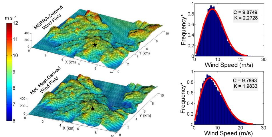
Fig. 1: Simulated mean wind speed for Case 1 scaled by measured (bottom left) and virtual climatology (top left) time series. Also, corresponding wind speed frequency distribution for the measurement location, as denoted by the black star, extracted from the model solutions scaled by the measured (bottom right) and virtual (top right) climatology time series.
