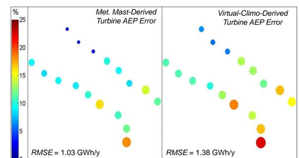
Fig. 3: Turbine specific, AEP error of Case 1 when CFD simulation is scaled by 50m met mast measurements (left) and virtual climatology (right). RMSE is computed using historical power production data as truth.
