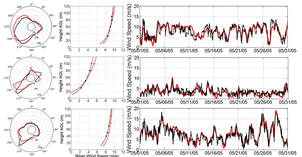
Fig. 2: Comparison of wind rose (left column), mean wind speed profile (middle column), and sample 50m wind speed time series (right column) for met mast location. Red represents virtual climatology and black represents measurements. The three rows correspond to cases 7, 2, and 4 (in order from top to bottom).
