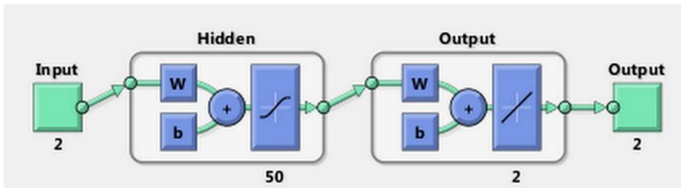
Fig. 1: Schematic showing the configuration of the feed-forward neural network used in this study. The inputs to the trained network are wind speed and direction from the reference time series and the outputs are predictions of the target time series.
