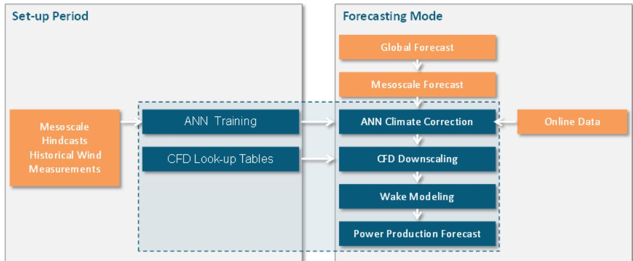
*Fig. 1: WindSim Power Forecasting Add-on module: Coupling procedure between meso- and microscale models. The parts in blue are processed inside the module and the parts in orange are data for training and running the module.*
