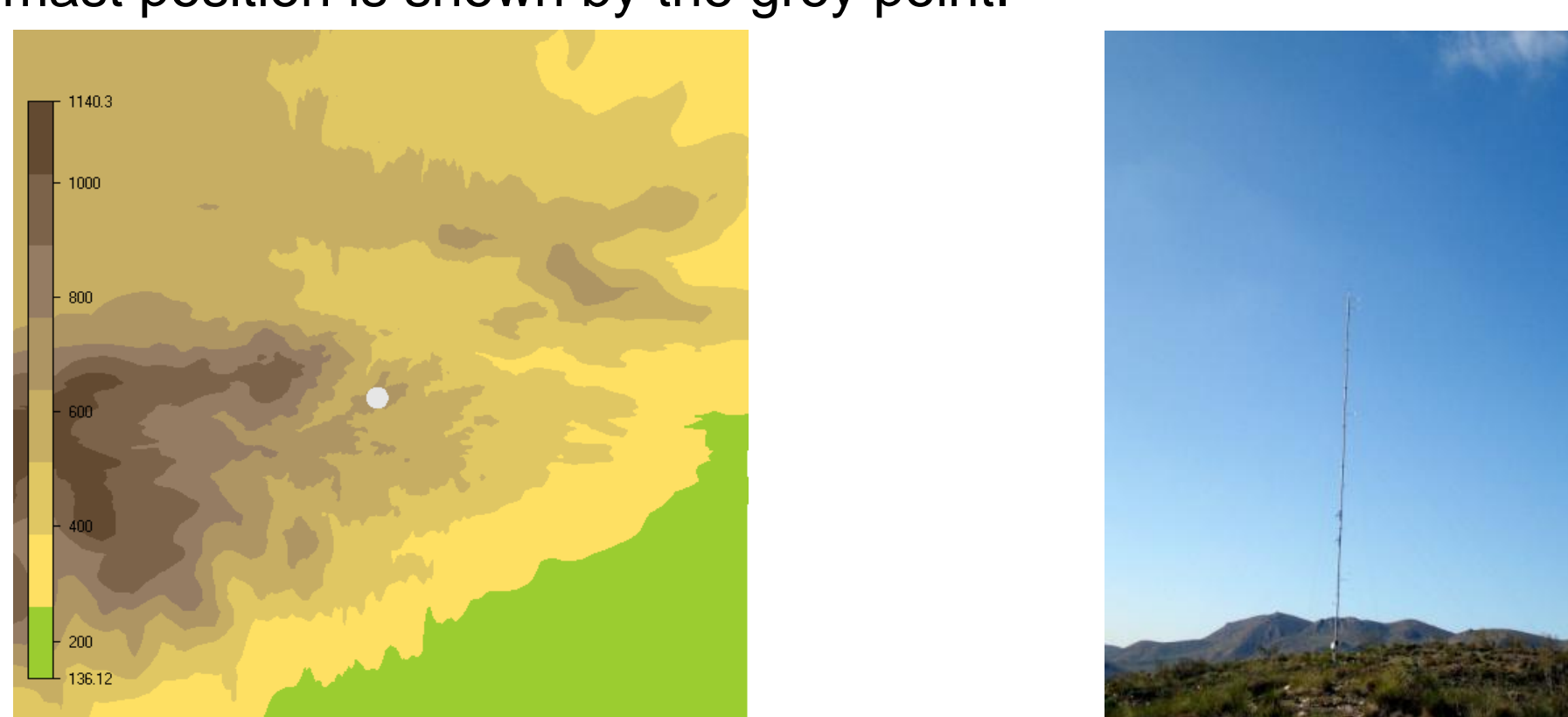
Fig. 4: Terrain height for Site 2. The measurement mast position is shown by the grey point.
